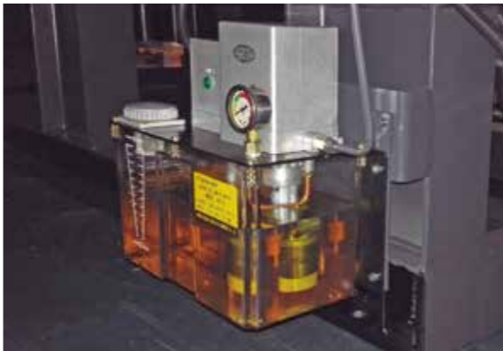
Automatic lubricating system The clamping unit is optimized for precise lubrication of all moving parts
