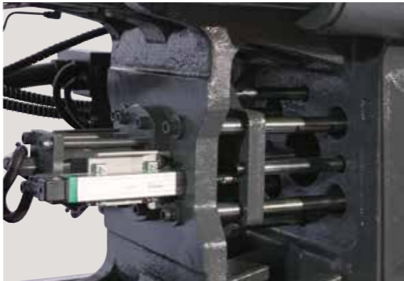
Multi-point Ejection System A great advantage for molds with different ejection requirements
